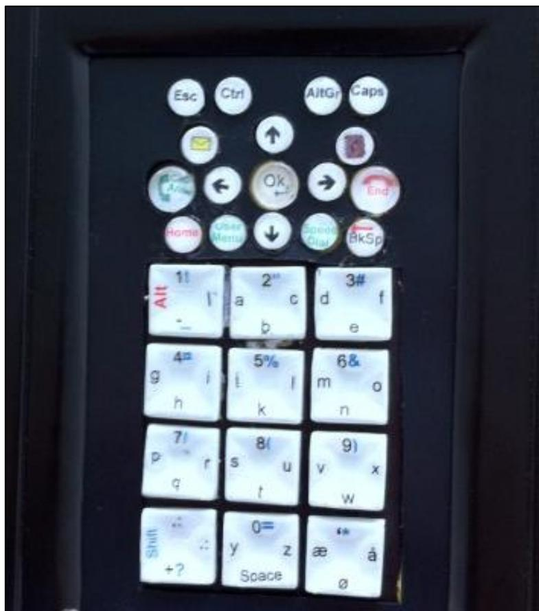
Figure 3 The prototype JusFone keyboard.
