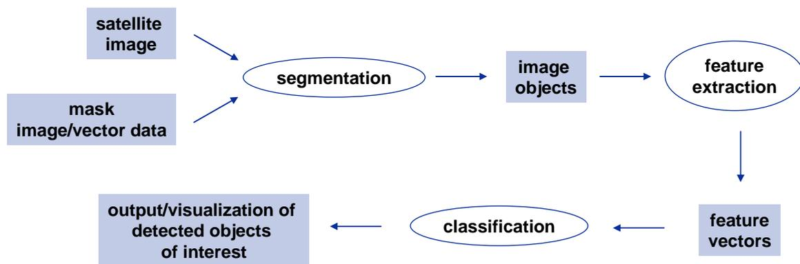
Figure 2-1. Processing flow of the general approach.
