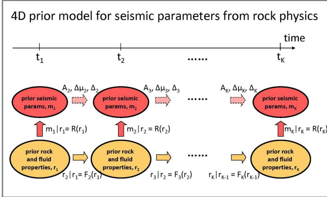
Figure 1 Seismic 4D prior from rock physics. The Markov property for rock physics parameters is shown with yellow arrows, the locality in time in the relation between seismic parameters and rock physics parameters is shown by red, vertical arrows. The implied Markov property for the seismic parameters is indicated with dashed, faint red, horizontal arrows.
