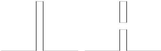
Figure 7: Illustration on how a removal of a pixel may result in an illegal configuration.
