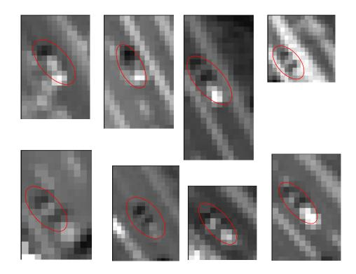
Manually identified vehicle objects that are not properly segmented. These objects have a low contrast to the background and are therefore fragmented into several very small parts.
