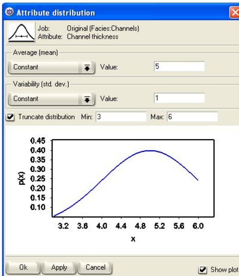
Figure 1: The RMS panel used to set parameter in truncated distribution for channel thickness.
