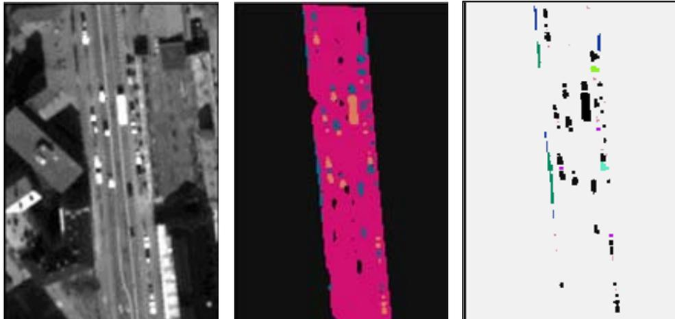
**Figure 3:** Result of the segmentation on a part of the road from the GO subimage. **Left:** Grey level image, **Middle:** Segmented road surface (pink), dark objects (blue), bright objects (orange) and not within mask (black). **Right:** Result of pre-classification, where the regions that are black correspond to objects identified as potential vehicles.
