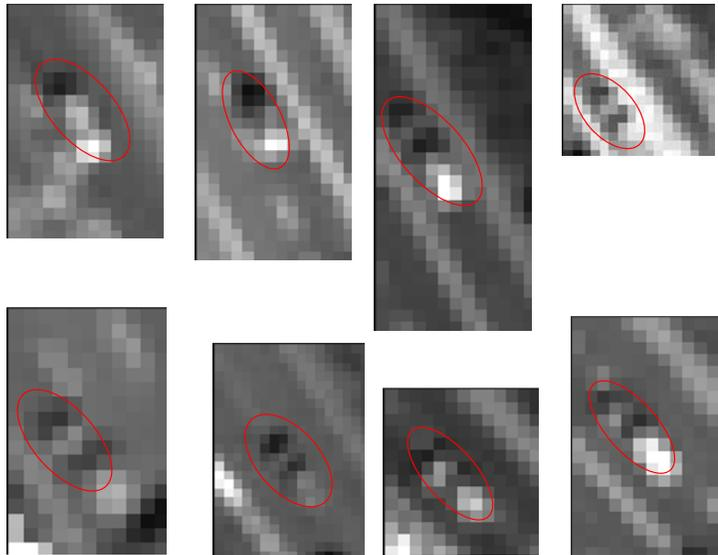
**Figure 4:** *Examples of manually identified vehicle objects that are not properly segmented. These objects have a low contrast to the background and are therefore fragmented into several very small parts that are not sufficiently large to be considered as a potential vehicle.*
