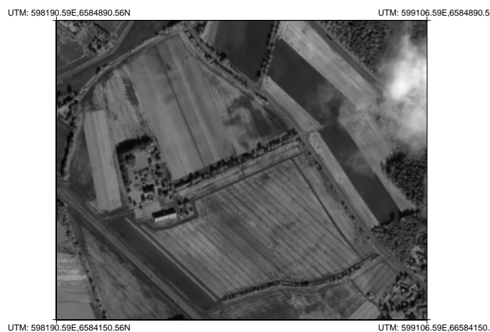
Figure 4: The Gipsund farm and the surrounding fields, panchromatic IKONOS data (1m resolution). The scene comprises 741 rows of 917 pixel for a total of 679497 pixels. The delimiting UTM coordinates are given in the corners of the image.
