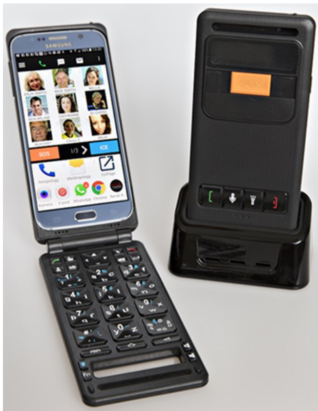
Figure 1. The EziSmart solution: To the left, the Ezi-Pad case is flipped open, providing access to the smartphone screen and the Ezi-Pad keypad. To the right, the case is closed and placed in the accompanying charging dock.
