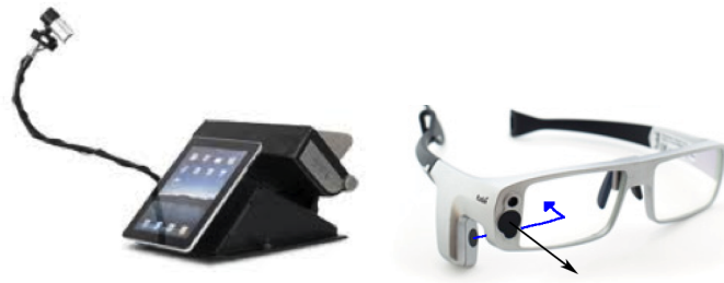
Figure 13. Eye trackers; stationary system (left) and as eye glasses (right)
