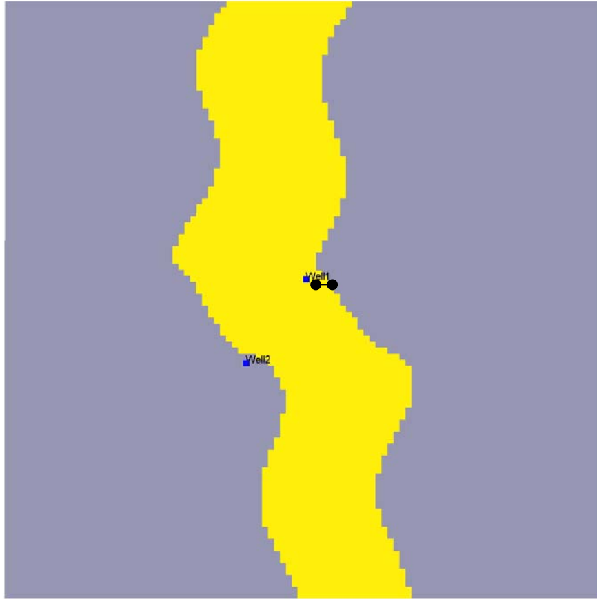
Figure 6: Channel conditioned on positive observation in Well 1 with distance limitations for nearest edge. Negative observation in Well 2
