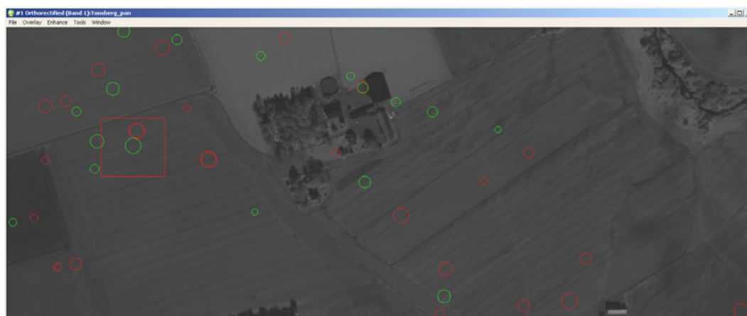
Figure 49. Detail of processed image with detections, corresponding to the red rectangle in Figure 48. Note the apparent random scatter of detections and the presence of circular and sub-circular features.
