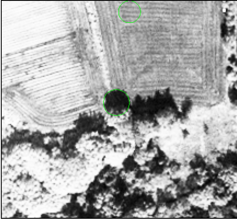
Figure 71. Hedrum no 18. Negative detection made by CultSearcher. The object is a three and its shadow into the cultivated field.
