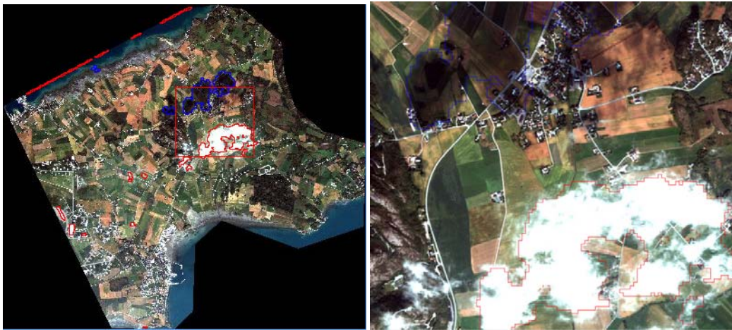
Figure 6-20: Left Image: Cloud/shadow map of the Ørland August 7, 2004 Quickbird image. Red lines indicate detected clouds, and blue lines indicate detected cloud shadows. Right image: Zoom indicated by the rectangle.
