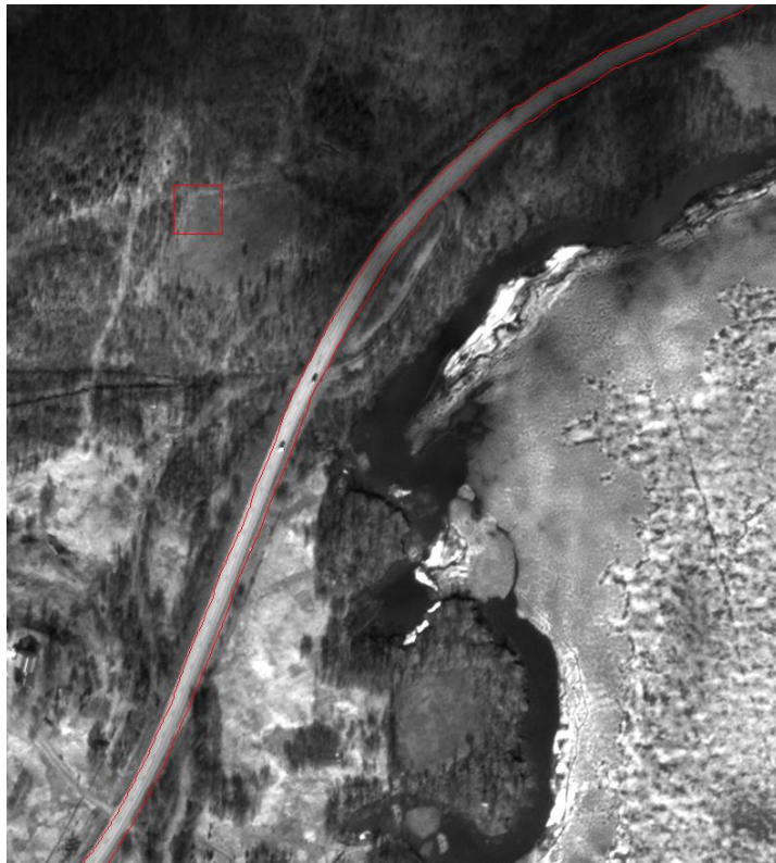
Figure 6-16: Part of segmented road after panchromatic refinement.
