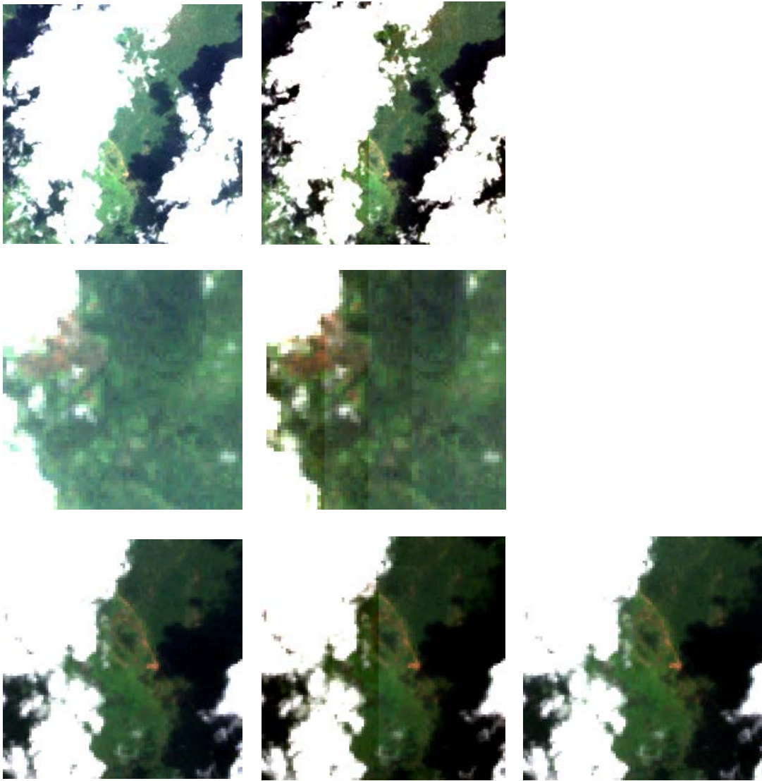
Figure 5. Details of a Landsat 7 ETM image over Tanzania on January 15, 2001. Left column: original radiance image. Middle column: surface reflectance image after atmospheric correction with FLAASH. Right column (only one image): surface reflectance image after atmospheric correction with FLAASH. Right column (only one image): surface reflectance image after atmospheric correction with LEDAPS.
