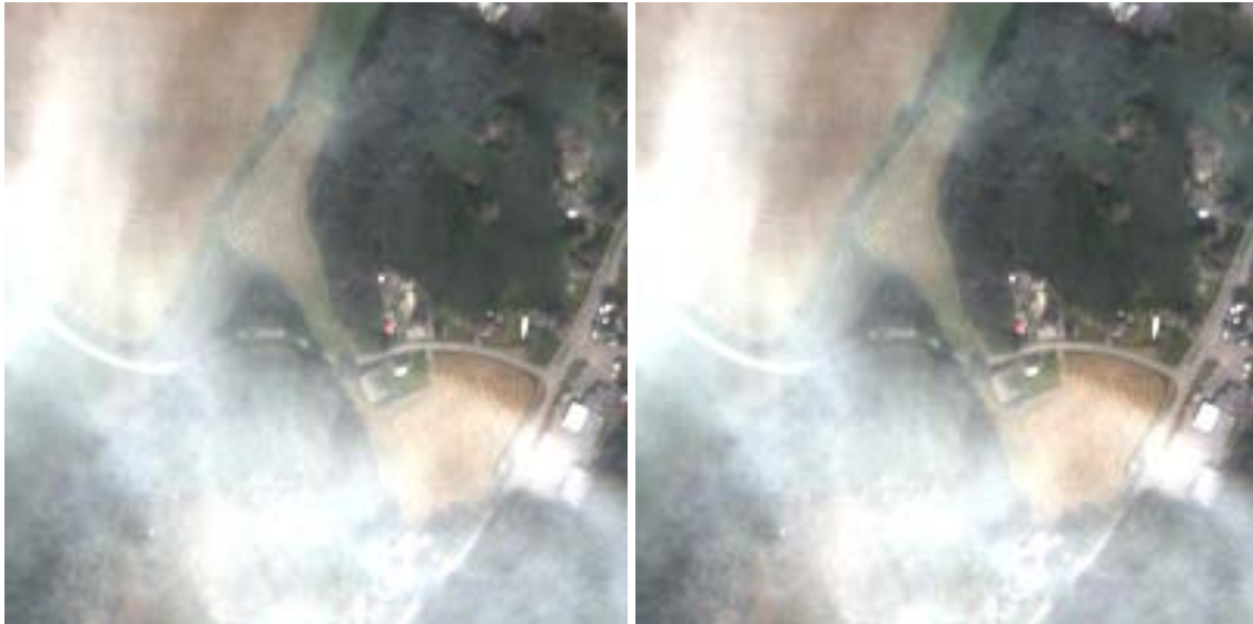
Figure 12. Tjølling, July 24, 2009. RGB composite using QuickBird bands 3, 2 and 1. Left: Original calibrated radiance image. Right: Surface reflectance image after FLAASH atmospheric correction.
