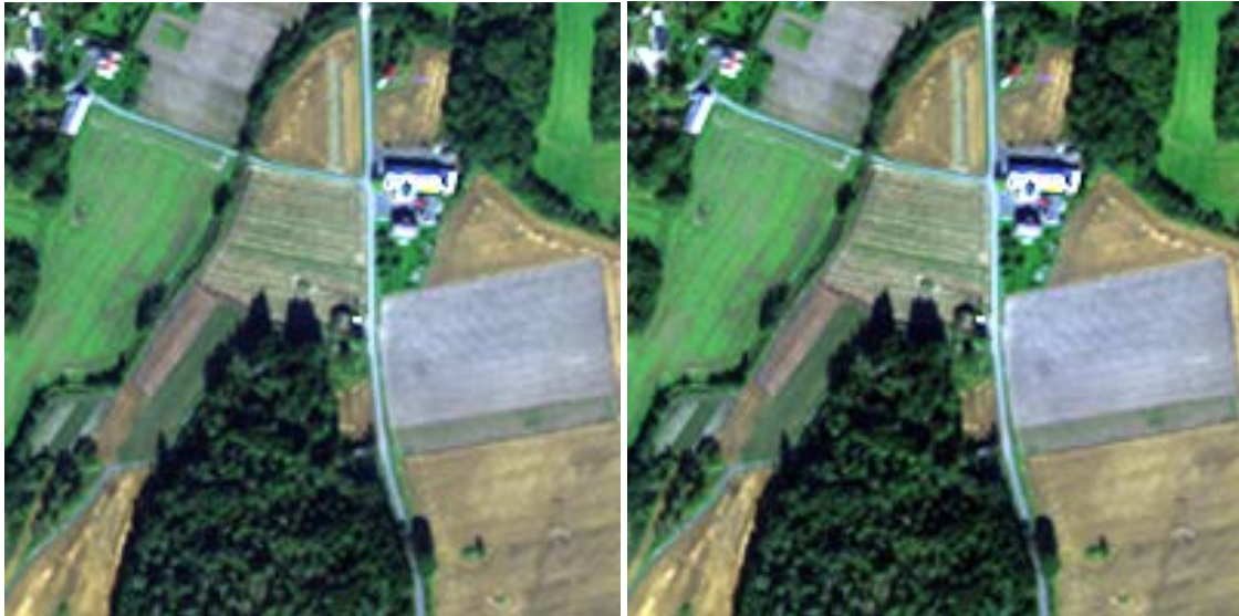
Figure 15. RGB composite of Worldview-2 bands 5, 3 and 1. Left: original image. Right: image after atmospheric correction with FLAASH.
