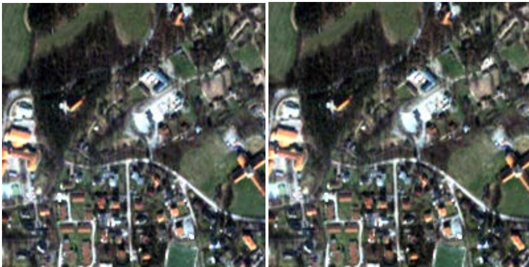
Figure 10. Oslo, May 5, 2006. RGB composite using QuickBird bands 3, 2 and 1. Left: Original calibrated radiance image. Right: Surface reflectance image after FLAASH atmospheric correction.
