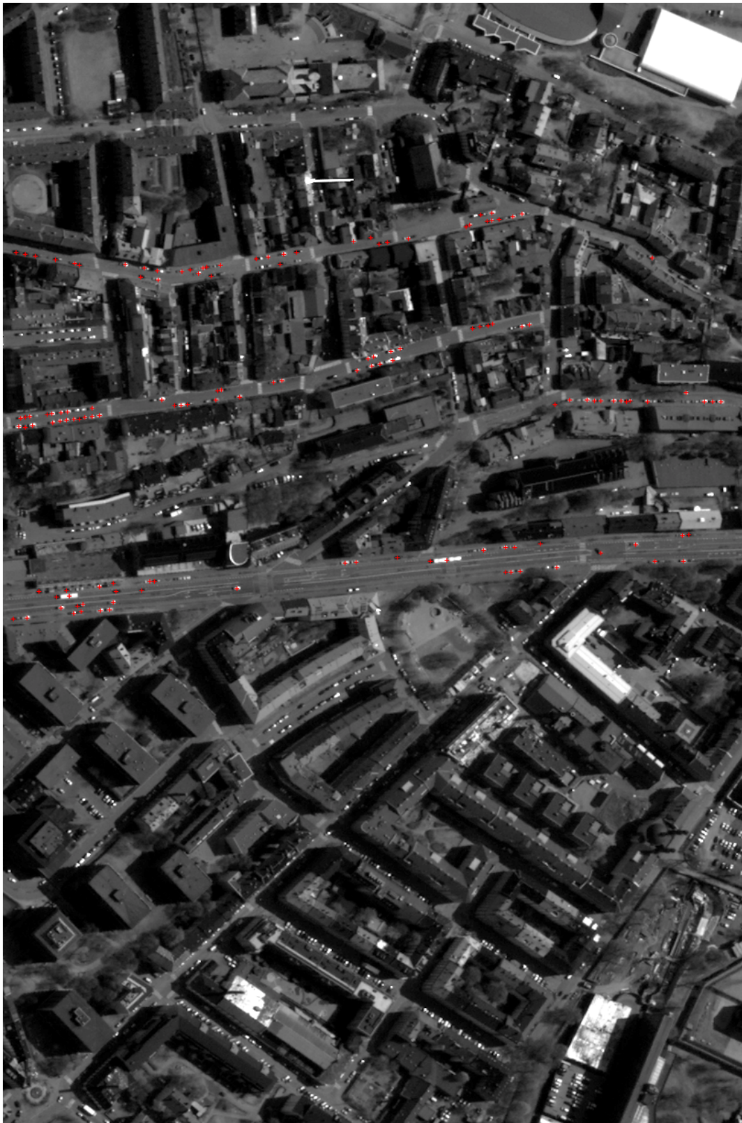
Figure 19: Base product for part of the SCA. This figure shows the vehicles detected by the system as red crosses, it is a larger version of the image shown in Figure 18 b). Notice that compared to Figure 18 b), this version of the image is rotated 90 degrees counter-clockwise.
