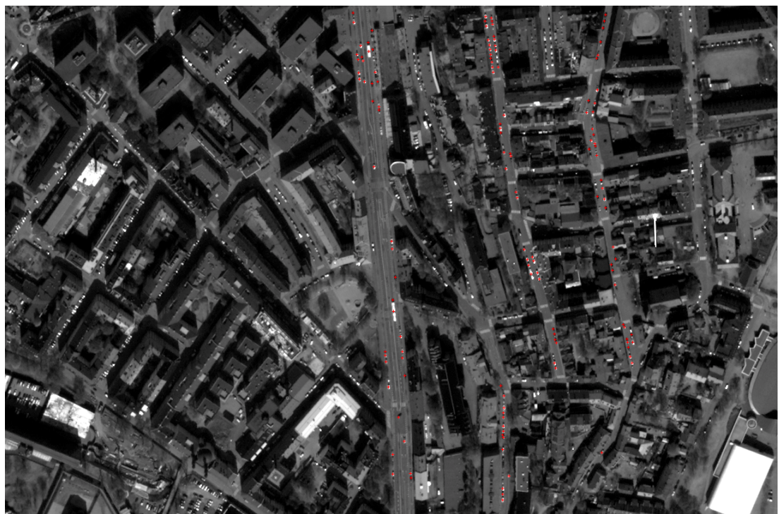
Figure 18: Base product for part of the SCA. Part a) of this figure shows the SCA as seen in the 2006 satellite image. The road masks used in this image are also shown. Part b) of this figure shows the vehicles detected by the system as red crosses.
