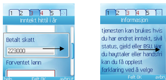
Fig. 2. Elastic scroll bar showing the relative position.
