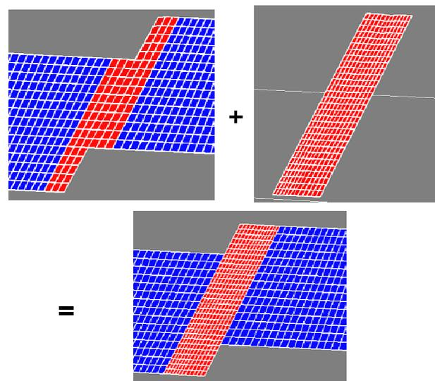
Figure 1: Merging of coarse and fine grid.
