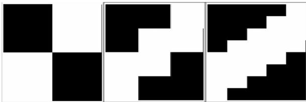
**Figure 3: Fault Product Distribution Factor with one, two and four slip planes symmetrically located in the fault zone. Slip planes are here simplified as having uniform displacement and spacing. The fault zone is mapped to a unit square.**
