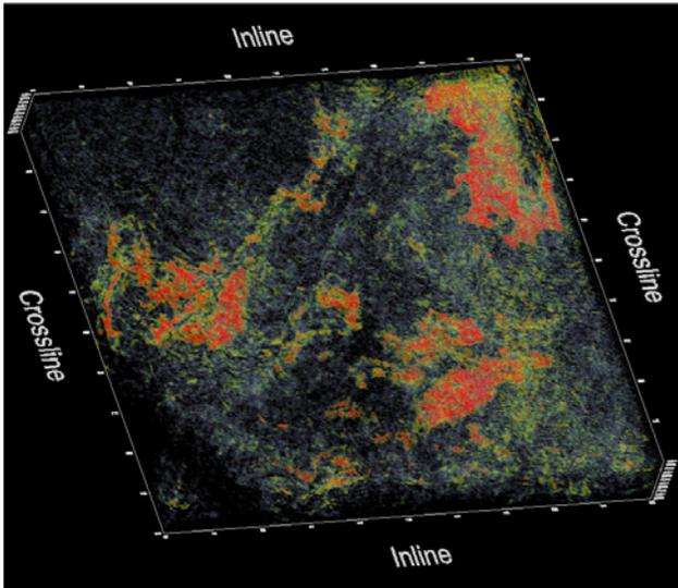
**Figure 3: Seismic far offset stack amplitude rendering indicates hydrocarbon saturated structures in the Alvheim area.**
