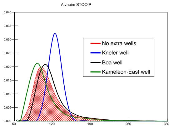
**Figure 9: Effect on STOOIP for a large Kneler oil column discovery, a medium Boa oil column discovery and a small Kameleon-East oil-column discovery.**
