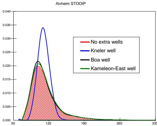
**Figure 8: Effect of a discovery of expected oil column for each of the structures on STOOIP.**
