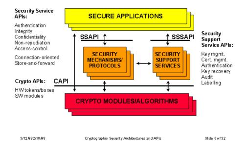
Figur 4.0:Basic layered cryptographic security architecture
