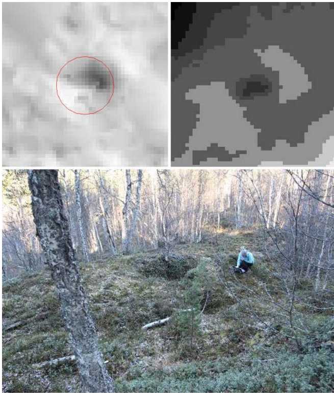
Figure 7. A small pitfall trap in the Olstappen training set. This pit was not found during the initial visual inspection of the laser data, but detected by CultSearcher, and confirmed in the field. Upper left: hill-shaded relief image. Upper right: elevation image, 0.3 m height resolution. Bottom: field image.
