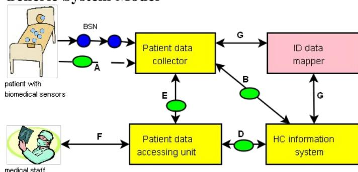
*Generic System Model with components (boxes) and channels (arrows). The green markers denote channels that must be protected.*
