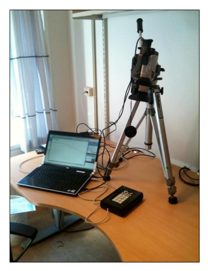
Figure 6 The set up for testing the JusFone keyboard.
