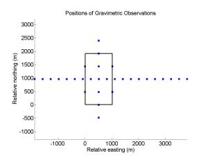
Figure 9. Observations points marked with blue relative to outline of reservoir. Note that most of the observations points are outside the region that is right above the reservoir.
