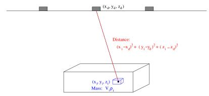
Figure 1. Sketch of reservoir, sea bed and gravimetric observations points.
