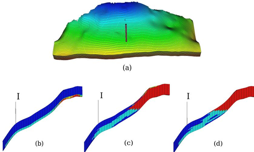
Figure 2: (a) Model geometry and well position. Model dimensions are  $3\text{km} \times 9\text{km} \times 80\text{m}$  with 20 layers. The bottom row shows the side view of  $\text{CO}_2$  distribution (in red) at the end of simulation in different aggradation cases, from low (b) to high (d). The vertical direction is exaggerated.
