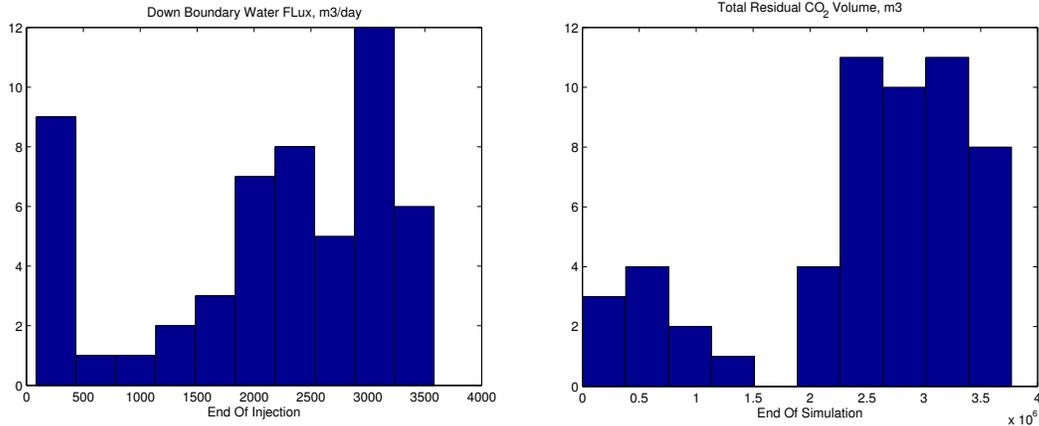
Figure 4: (a) Flux histogram for down boundary: cases with low aggradation show high values. (b) Total residual CO<sub>2</sub> volume; cases with low aggradation show less values in a separate family.
