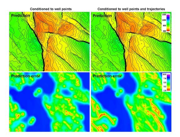
The two upper figures are the predicted depth to the surface and the two lower figures are the corresponding prediction errors. The change in the predicted depths are subtle in this case but the prediction errors has been significantly reduced along the well paths.
