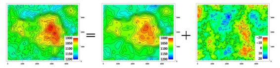
The trend can be a single known map or a linear combination of many known maps. The trend determines the main shape of the surface so the choice of trend maps is very important. The residual is usually small compared to the trend. The residual is specified by an residual uncertainty (standard deviation) and a spatial continuity determined by a variogram. The residual is in principle unknown and random.
