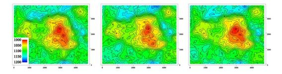
The average of a large set of simulations will coincide with a prediction. The standard deviation of the large set of simulations will coincide with the prediction error.
