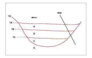
Figure 8.4. Zones where surface TD is on-lapped. The well points are given as green bullets.
