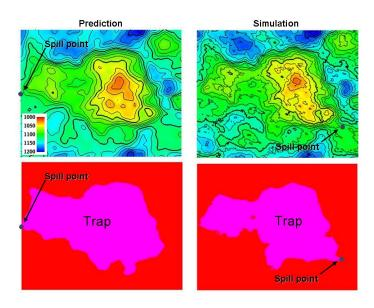
The spill point is detected and written to file (x-, y-, and z-coordinate). Also the trapped area can be written to an output grid file. Note that the spill point for the predicted and the simulated surfaces can be quite different.
