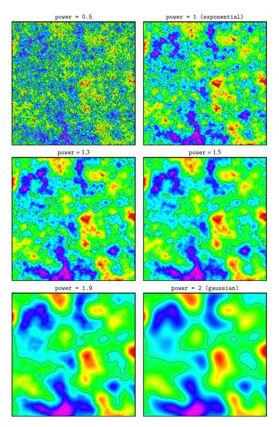
Figure D.2. General exponential variograms for different power>. Note that the exponential variogram is identical to power = 1 and the gaussian variogram is identical to power = 2.
