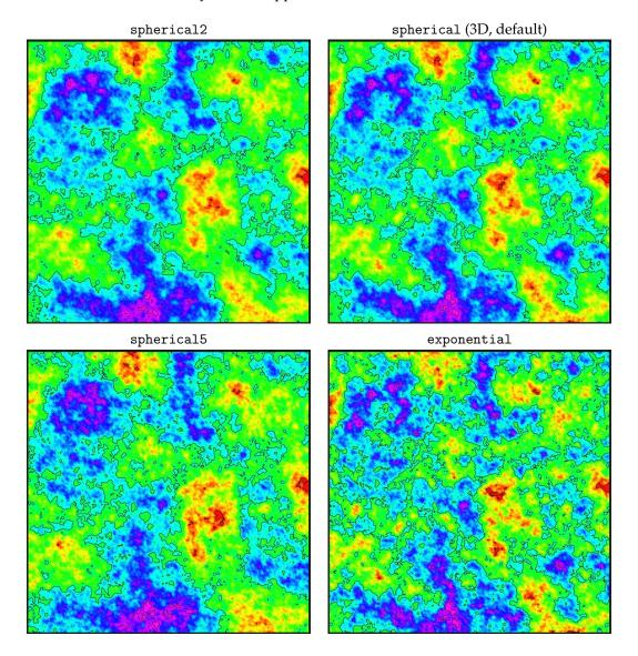
Figure D.1. Spherical and exponential variograms.
