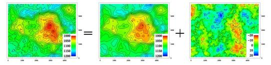
The trend is obtained from a seismic travel time map and a model for the interval velocity trend. The residual is a simulation of a possible realization of the mismatch between the trend and the real depth to the surface.
