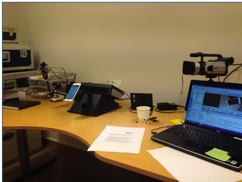
Figure 4: The setup for the testing environment. The phone is fixed to a stand with a web camera looking at it. Another camera is positioned to film the face. The cameras are fed into the computer running Morae in the right corner of the figure.
