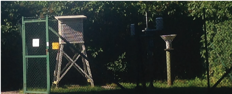
Figure 2. Thermometer and other instruments at Stockholm Observatory, where measurements have been made daily since 1756. The station has been moved short distances twice during this time. The box to the left is a Stephenson screen, and was used for the measurements until 2006. The pipe sticking up in the middle contains the modern measurement device that has been used since then.
