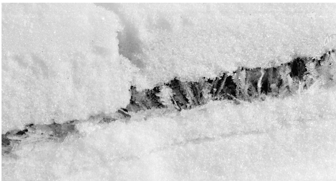
Figure 1.1. Fractured and collapsed (left) and unfractured, intact (right) part of a weak layer of buried surface hoar. Photo credit: ASARC (Applied Snow and Avalanche Research), University of Calgary Canada. By courtesy of Prof. B. Jamieson, ASARC.
