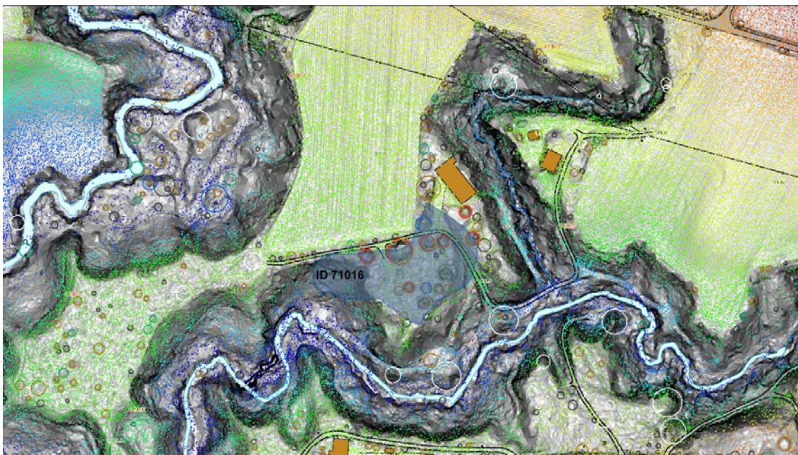
Figure 18. The grave field at Ødelund, with Askeladden site ID 71016. Blue shade: outline of grave field, according to Askeladden. Coloured dots: ALS ground points, with the colour indicating terrain elevation. Circles: automatic heap detections by CultSearcher, with red=high confidence, blue=medium high, green=medium, brown=low, black=very low, and white=zero confidence.
