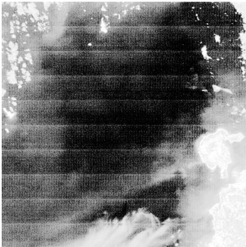
Figure 5 Part of NASA image from 29 May 2007, 0930 UTC. The gray scale has been adjusted to show the repeating patterns in the input values.
