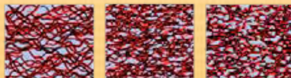
Figure 3: Markov mesh model. A training image to the left, a sample obtained using a Markov mesh model (middle), and a sample made by SNESIM (right). The simulated samples have a lot in common with the training image but they are generally more rugged.
