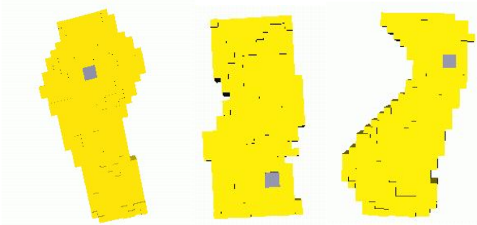
Figure 9: Backbone objects in GMPP conditioned on distance to well. Left: a=400 , b, c, d are missing. Middle: a=100 , b=200 , c and d are missing. Right: a=100 , b=200 , c = 250 , d=300 . In all cases, the mean object width is 600.
