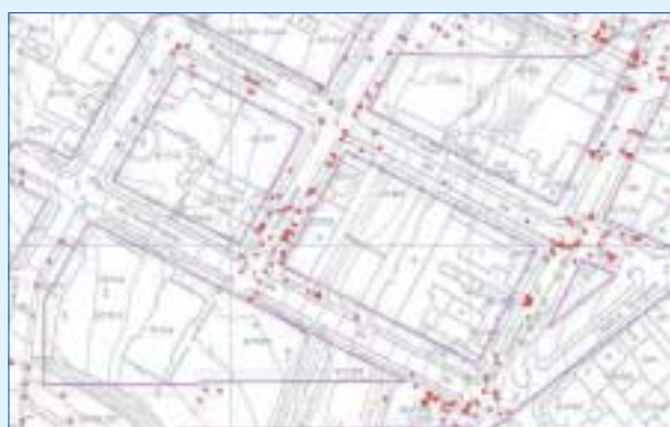
Instant detection of object classes at a telecom map by drawing a purple corridor across the map.
