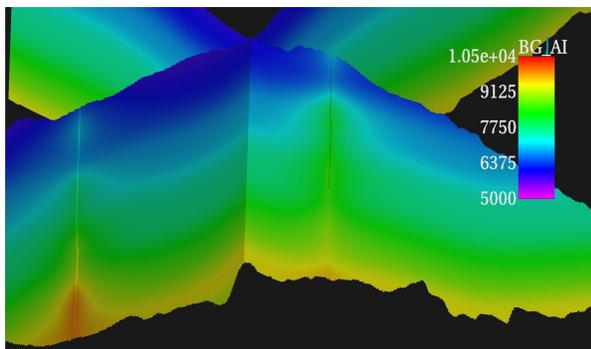
Figure 4: The background model for AI. Also shown are two AI well logs filtered to 6 Hz.
