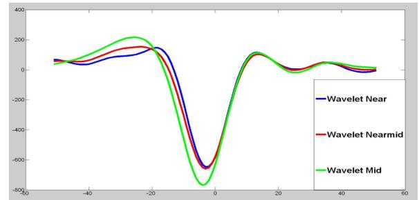
Figure 2: The estimated wavelet for different angular stacks.
