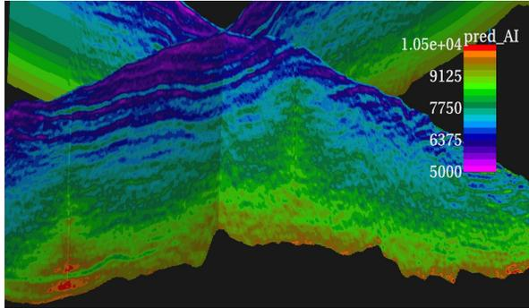
Figure 3: Cross sections of the predicted AI. Also shown are two AI well logs filtered to 40 Hz.
